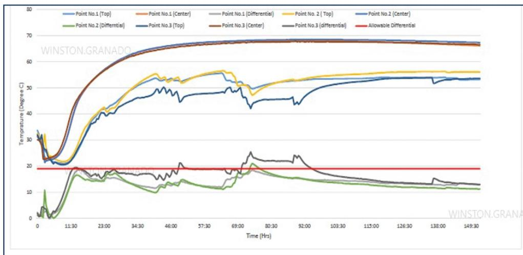
Figure 5: Temperature Report on Compressor Foundation No. 1 [6]
