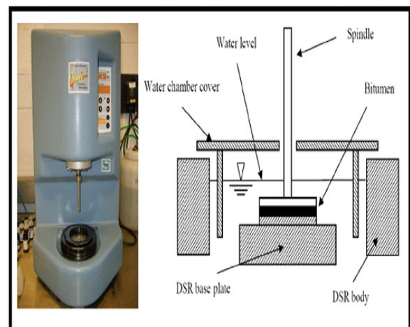
Figure 3: Schematic of dynamic shear rheometer testing configuration [33]
