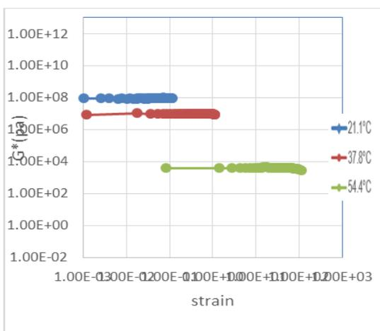
**Figure 9:** Linear Visco Elastic Range for 5% Modified Binder ARTFO
