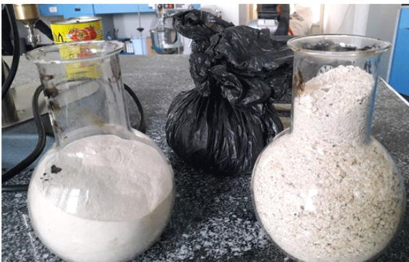
**Figure 1:** Sample preparation for Portland cement and Waste Animal Bone powder
