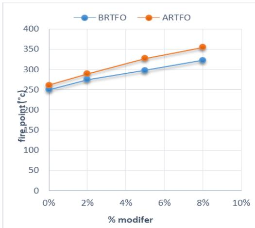
**Figure 8:** Fire point test result
