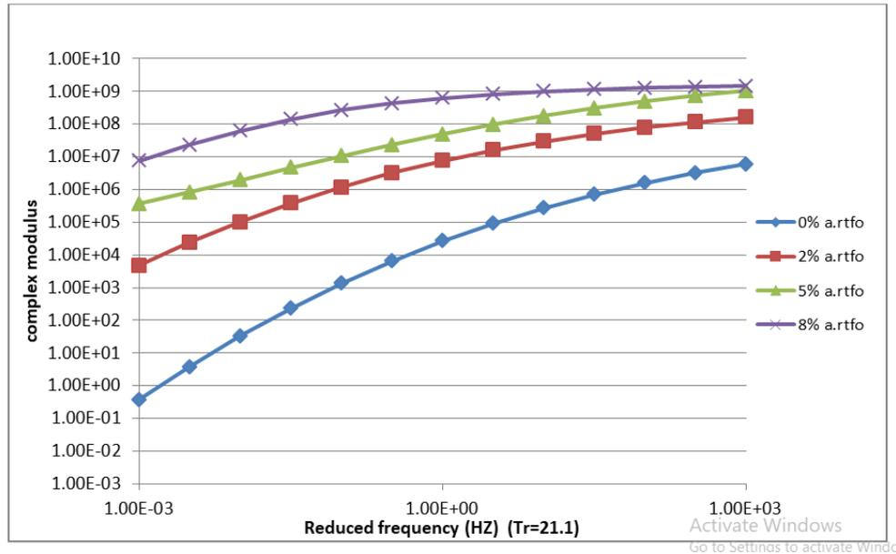
Figure 11: Complex Modulus master curve
