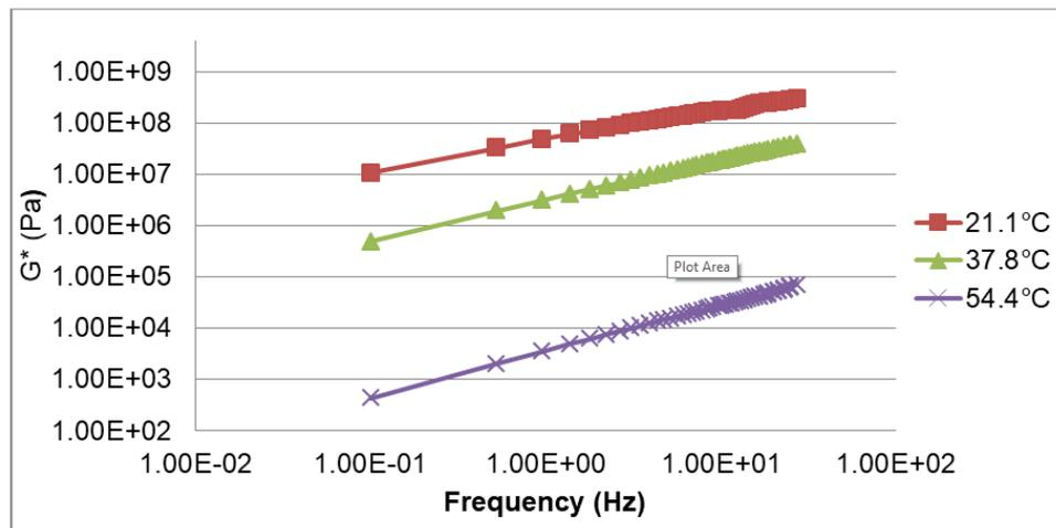
**Figure 10:** Frequency Sweep Test Result 5% PCWAB After RTFO
