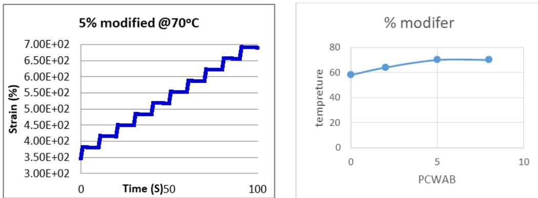
Figure 12: Addition of Portland cement and waste animal bone improves Rutting resistance at high temperature
