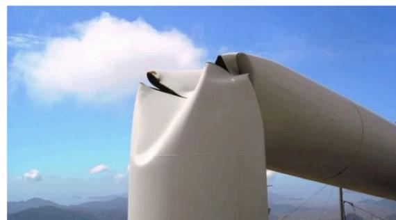
**Figure 1:** Collapse of steel tower due to local buckling
