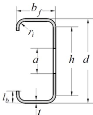
**Figure 1:** Typical sectional profile for lipped channel sections with holes
