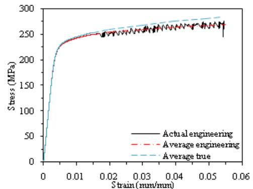
**Figure 2:** Typical stress-strain curve for 5052-H36
