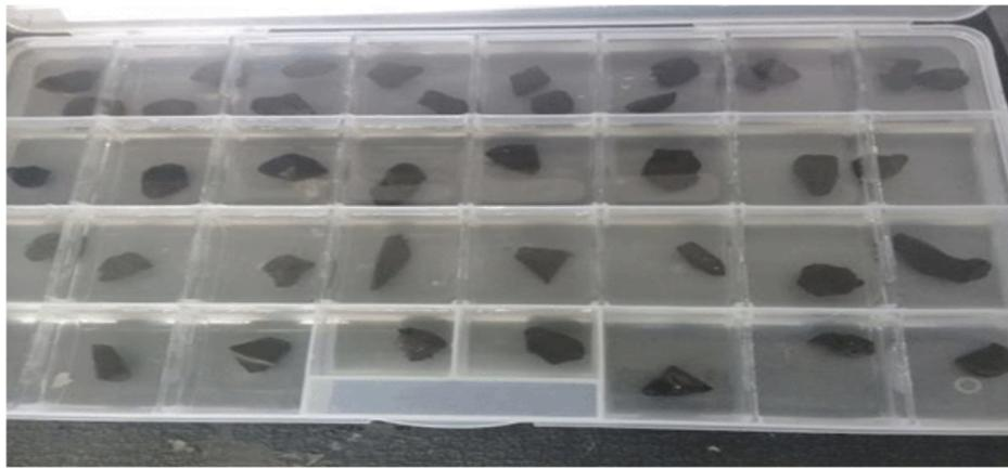
**Figure 1:** Slag soaked in Ethylene Glycol
