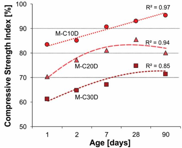
**Figure 8:** Compressive strength index of mortars
