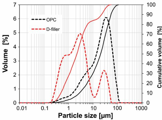
**Figure 3:** PSD and cumulative volume curve of OPC and D-filler
