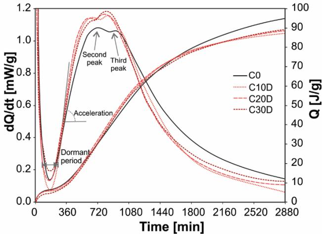
**Figure 4:** Heat release rate and cumulative heat for D-filler pastes
