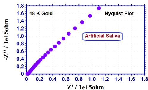
**Figure 4:** AC impedance spectrum of 18 K Gold immersed in Artificial Saliva
