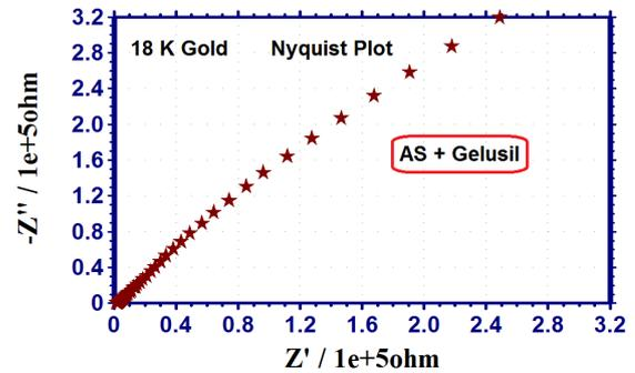
**Figure 6:** AC impedance spectrum of 18 K Gold immersed in Artificial Saliva (Nyquist Plot)
