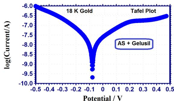
**Figure 2:** Polarization curve of 18 K Gold immersed in artificial saliva in the presence of Gelusil
