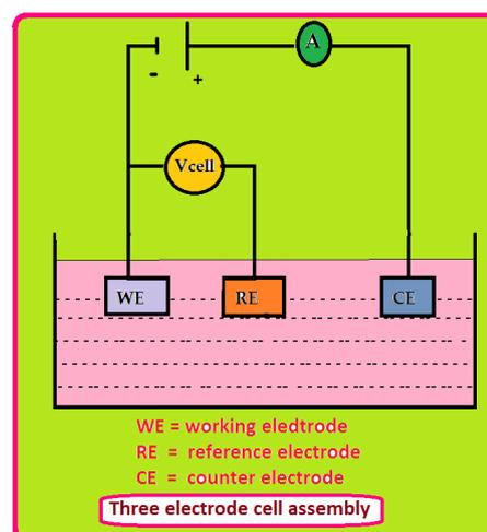
Scheme A. Three electrode cell assembly
