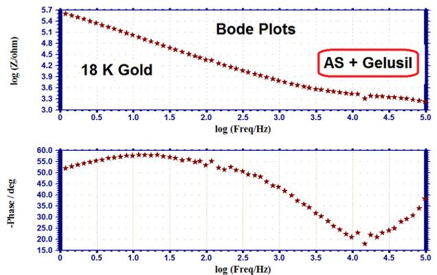
**Figure 7:** AC impedance spectra of 18 K Gold immersed in Artificial Saliva in the presence of Gelusil (Bode Plots)
