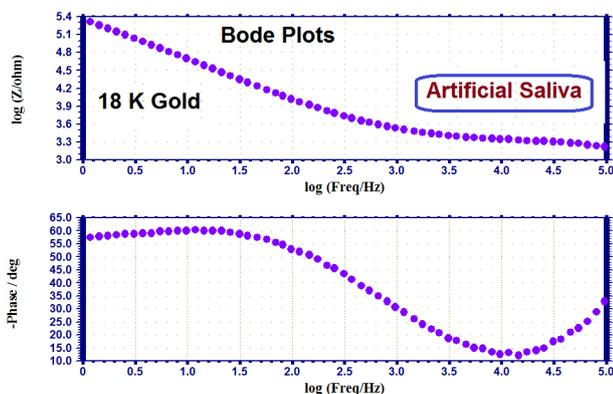
**Figure 5:** AC impedance spectrum of 18 K Gold immersed in Artificial Saliva in the presence of Gelusil
