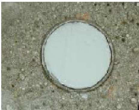
Figure 3: Adhesive L1 applied on the concrete surface
