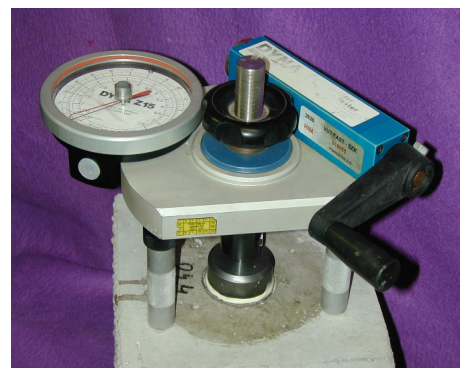
Figure 2: Pulling-off the target with DYNA Z 15
