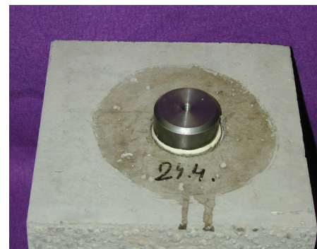
Figure 1: Gluing of the pull-off target to the substrate
