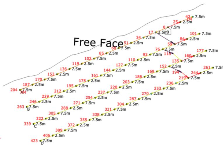
**Figure 4:** Delay sequencing of blast holes for excavation of composite strata using non-electric detonators.
