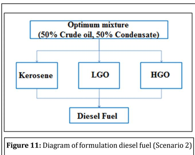
**Figure 11:** Diagram of formulation diesel fuel (Scenario 2)**Table 10:** Composition limit of blendstocks (Scenario 2)
