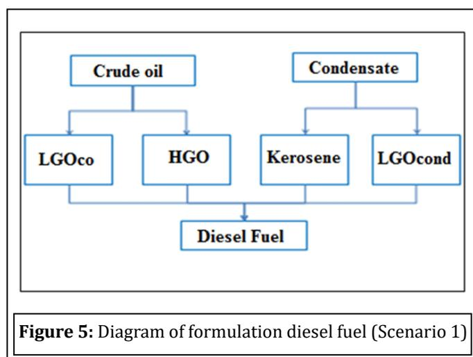
**Figure 5:** Diagram of formulation diesel fuel (Scenario 1)
