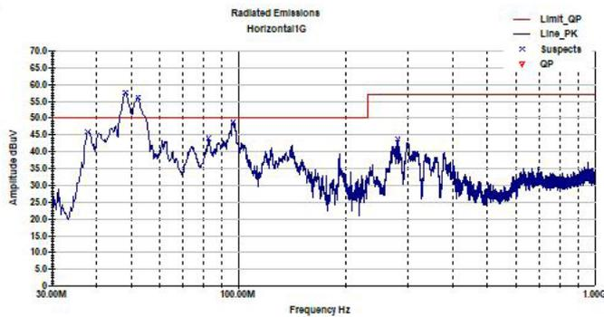
Figure 4: Far field radiation field during normal operation.
