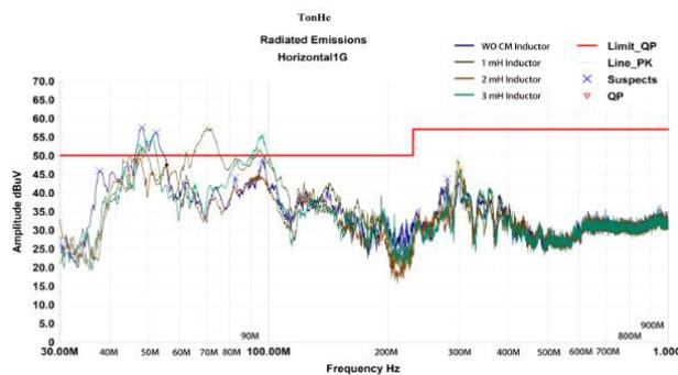
**Figure 8:** Effect of series common mode inductor on radiation (common mode inductor close to the load)
