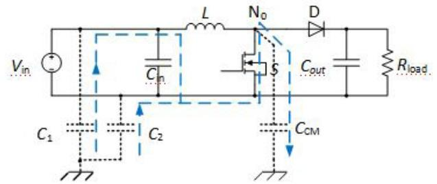
**Figure 2:** The Topology of Boost converter
