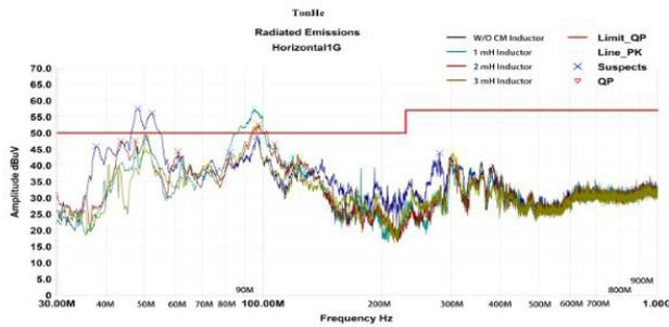
**Figure 7:** Effect of series common mode inductor on radiation (common mode inductor close to converter)
