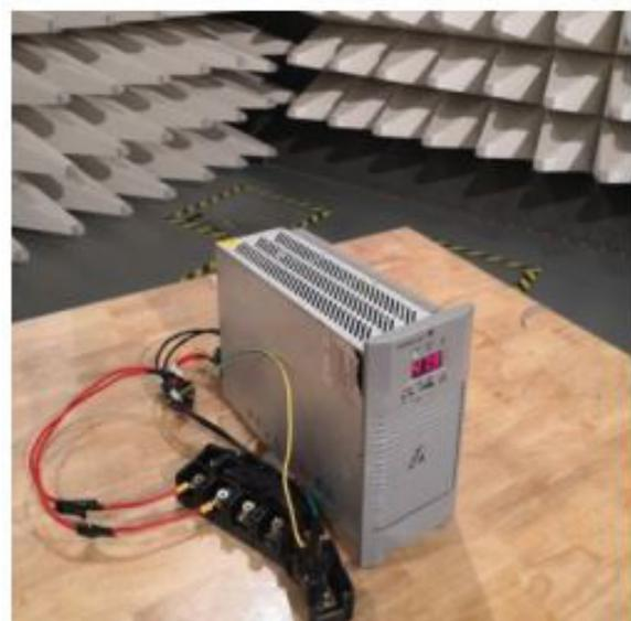
**Figure 3:** CM inductor connected to the near-end of converter module
