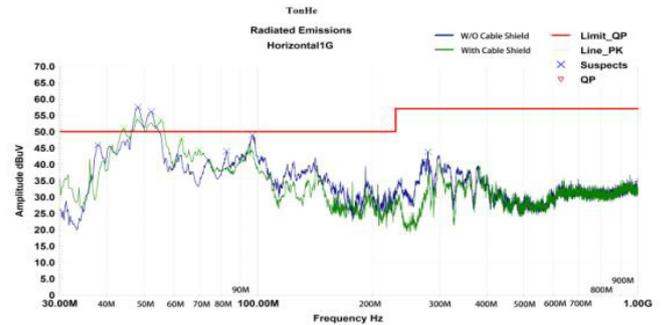
Figure 6: Effect of cable shielding on far-field radiation
