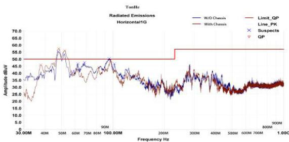
Figure 5: Effect of chassis on far-field radiation.
