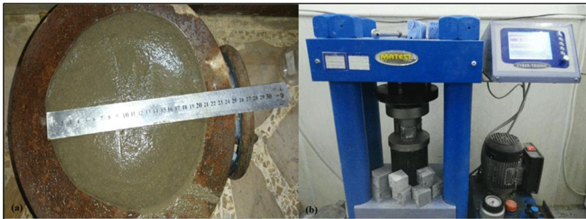
**Figure 1: Mechanical tests; (a) flow test and (b) compression test.**
