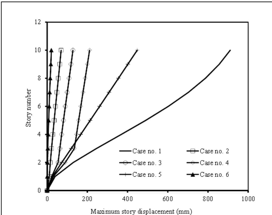
**Figure 5:** Story displacement in Y-direction
