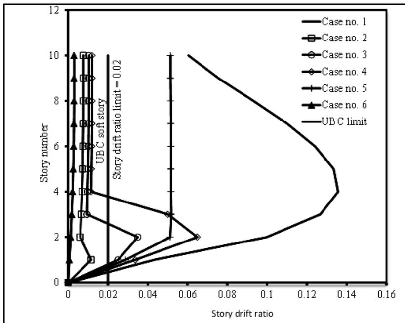
**Figure 9:** Story inelastic drift ratio in Y-direction
