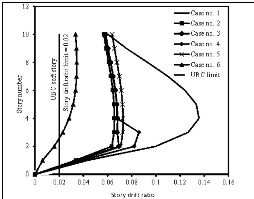
**Figure 8:** Story inelastic drift ratio in X-direction
