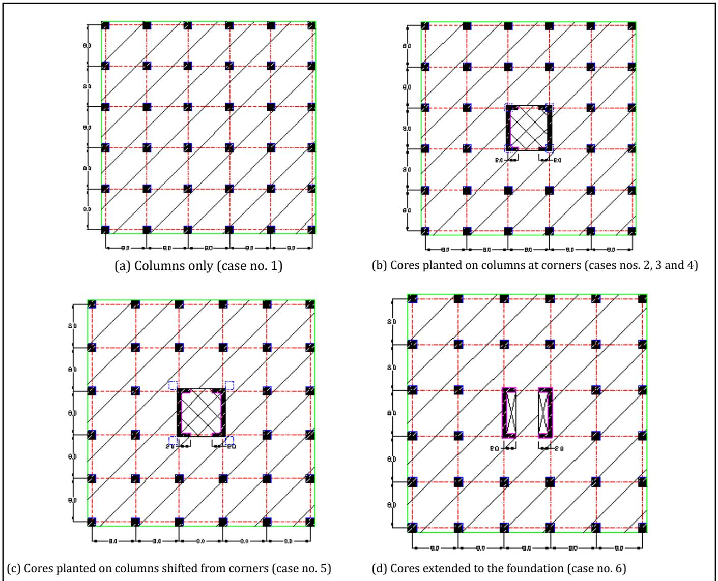
**Figure 1:** Building geometry
