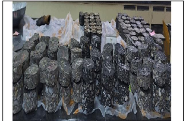
**Figure 4:** Part of the Core Specimens Obtained
