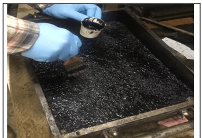
**Figure 5:** Tack Coat Application Process
