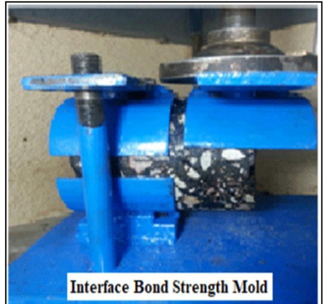
**Figure 7:** Interface Bond Shear Strength Mold
