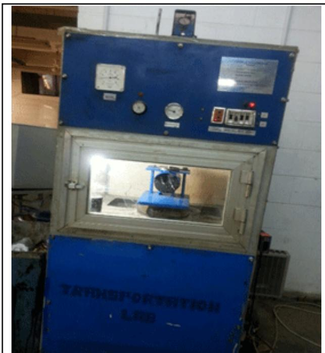
**Figure 6:** PRLS and the cyclic shear stress test
