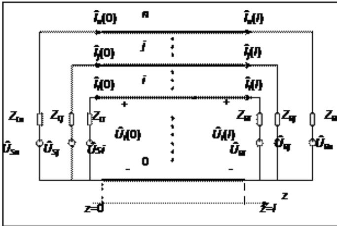
**Figure 1:** (n+1) conductor transmission model
