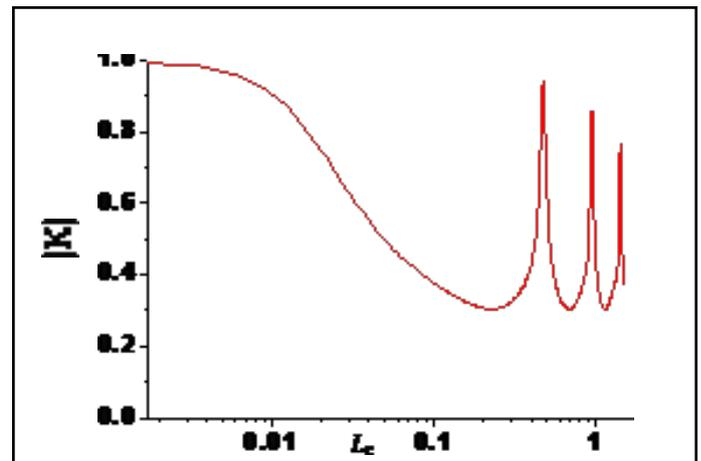
**Figure 3:** Interference line voltage transfer coefficient  $K$  of (2+1) transmission line
