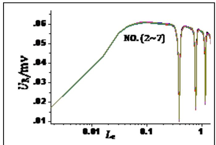
**Figure 6:** Far end crosstalk voltages of NO. (2~7) conductors
