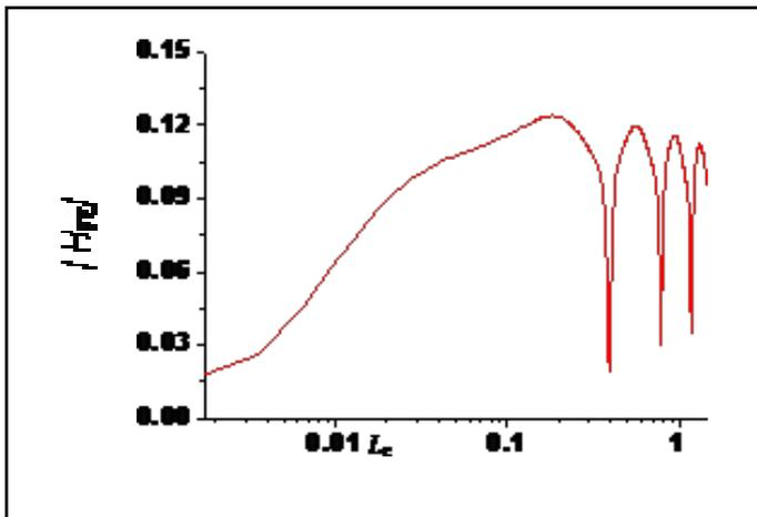
**Figure 8:** Far end crosstalk transfer function HFE of the (7+1) transmission line
