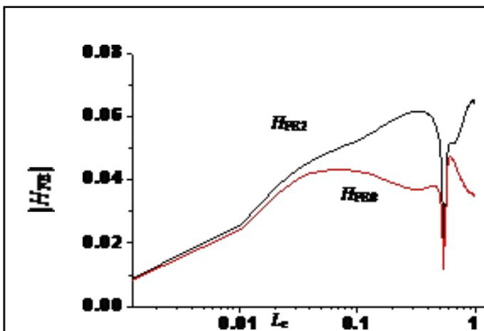
Figure 12: Far end crosstalk transfer function HFE of the (19+1) transmission line
