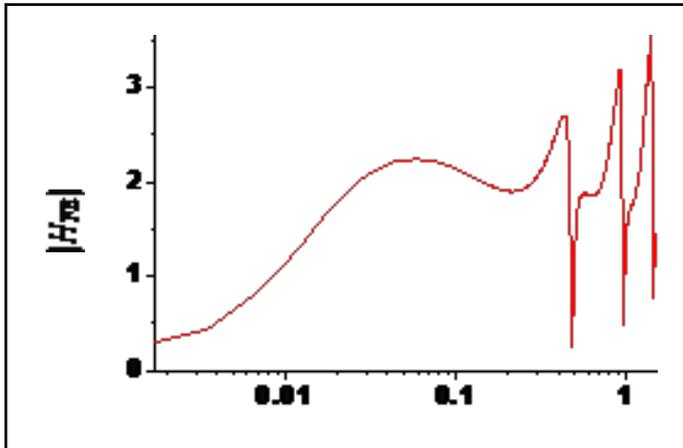
**Figure 4:** The far-end crosstalk transfer function HFE of the (2+1) transmission line
