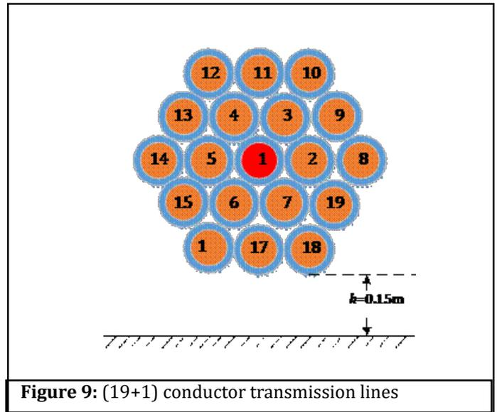
**Figure 9:** (19+1) conductor transmission lines
