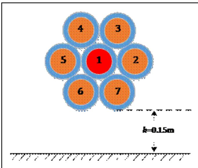
**Figure 5:** (7+1) conductor transmission lines
