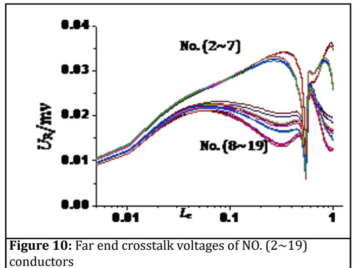
**Figure 10:** Far end crosstalk voltages of NO. (2~19) conductors
